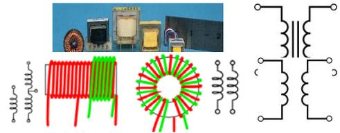
In both, the core is constructed of laminated sheets of steel to reduce eddy current losses. At high frequency, iron-core transformers suffer considerable power loss.
