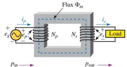
This ratio is called the **transformation ratio** (or the turns ratio) and is given by the symbol  $a$ .
