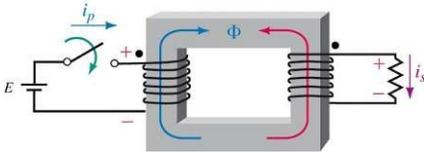
**Power Transformer Ratings** Just like ac motors and generators, power transformers are rated in terms of **voltage** and **apparent power**. For example, suppose a transformer is rated 2400/120 volt, 48 kVA.
