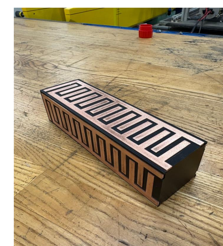
Machined and 3D Printed Inner TENG Piece
