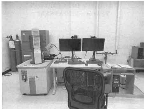
Figure 1. TESCAN MIRA3 SEM workstation in Ri237A. The gas bottles shown are nitrogen gas used for operating pneumatic valves in the SEM.
