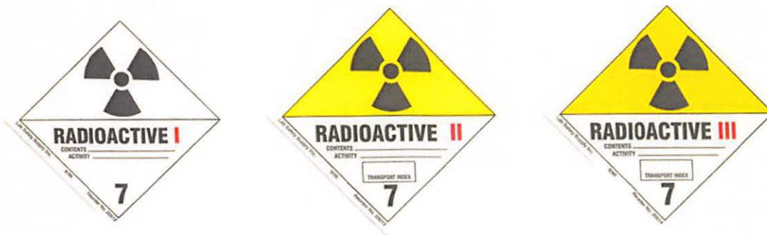
Figure 9-1 – Example of HAZMAT Labels
